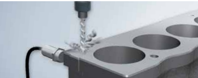
Position monitoring systems of machine tool with direct oil contact.
